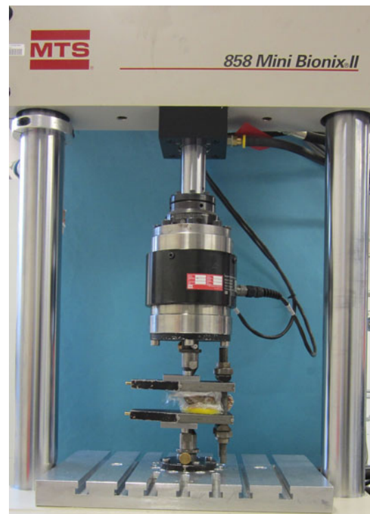
Fig. 1 The test setup in the material testing machine, with adjustable load application via ball-and-socket joints and a hinge joint at the dorsal side used to provoke a vertebral wedge fracture and for cyclic loading
